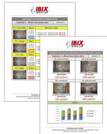
The 'PRINT REPORT' function included in the software that manages the **IBIX Mobile LAB** is used to create a comprehensive technical report of tests in PDF format, with a simple click of the mouse! The report shows charts and graphs with the results of the analyses carried out per sample; it includes the reference regulations and standards, test conditions, images to locate the collection points, and a guide to understand the readings.
