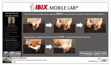
The dedicated software developed by START Apps S.r.l. controls all operations. It also guides the operator, step by step, on how to carry out chemical-physical tests in order to obtain objective results. These results will help designers, restorers and administrators of cultural heritage to devise a modern approach to conservation.
